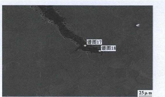
图 3 12Cr1MoV 钢 \Phi 500 mm 连铸坯典型缺陷形貌,SEM Fig. 3 Morphology of typical defects in \Phi 500 mm casting bloom of steel 12Cr1MoV, SEM
